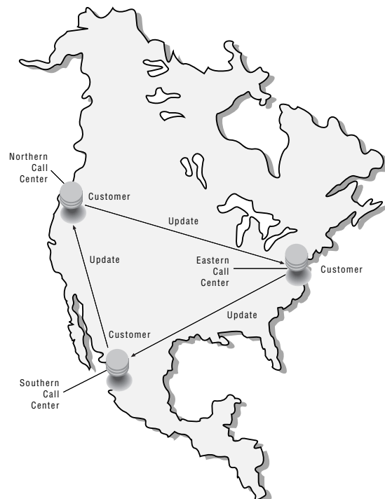
Figure 5. In an update-anywhere scenario, data may need to be owned and updated at some sites, while other sites have read-only copies.
